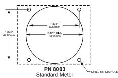
**Panel Mount:** For thicker mounting surfaces, the meter can be mounted into a 0.125" thick panel. Blue Sea Systems offers meter mounting panels for our standard size meters only. For PN 8003 use PN 8013 to mount a single meter or PN 8014 to mount two meters.
